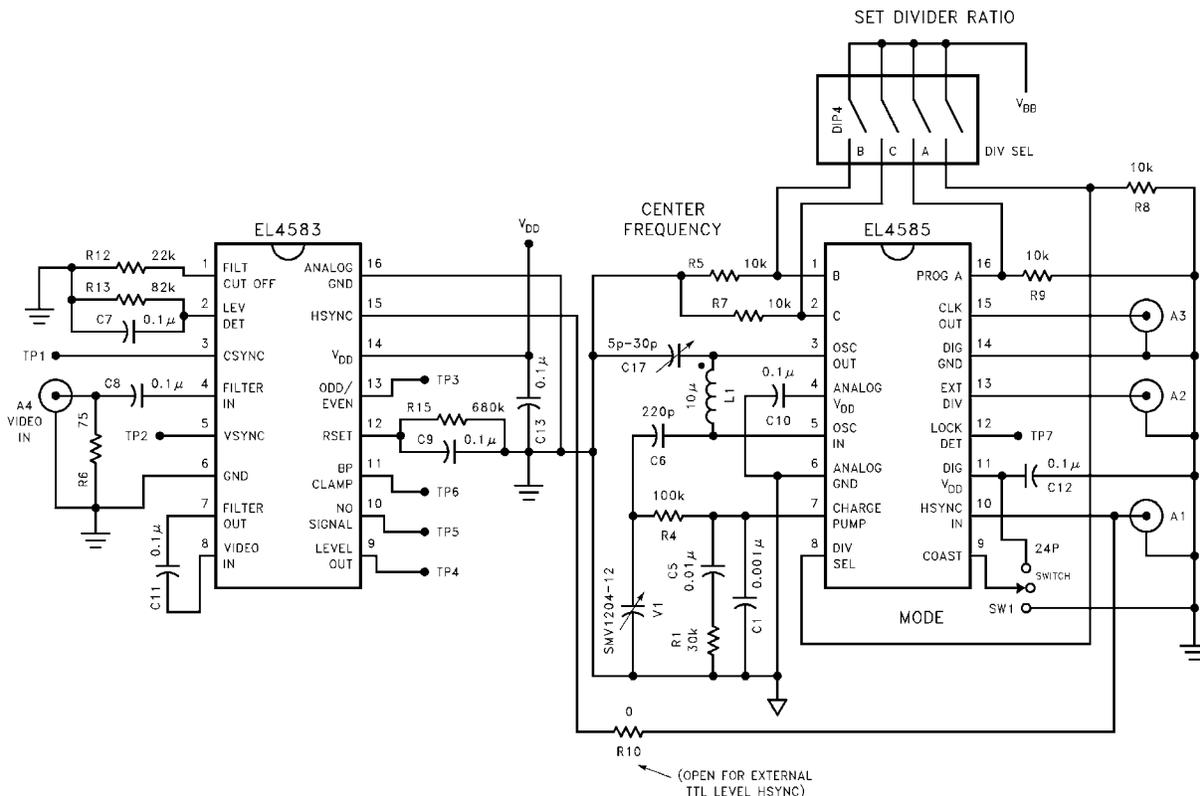
The VCO and loop filter section of the EL4583/4/5 Demo Board can be implemented in the following configurations:
