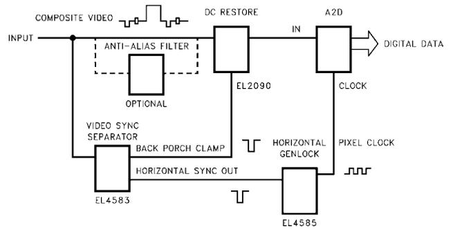
Horizontal genlock provides clock for an analog to digital converter, digitizing analog video.
